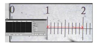
Enter the name of the calibration table created and the selected ruler length (the actual length). Assuming that the unit of dividing scale in the benchmark picture is  $\mu$ m, fill in the corresponding information at the designated place, as shown in the figure below: Click "Add" to add the benchmark defined in the benchmark picture to the calibration table in the software for subsequent operation.
