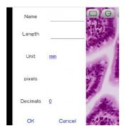
(3) Enter a name, the actual length of the calibration ruler, select a unit, and draw on the ruler, the pixels are automatically entered, as shown below. Click "OK" to complete the calibration.
